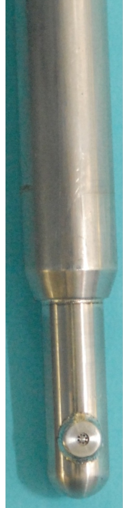
(b) Tip region of the probe after sealing and final welding.
