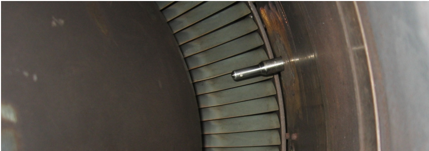
Figure 6.8: Photograph of the probe inside the Viper engine jet pipe
